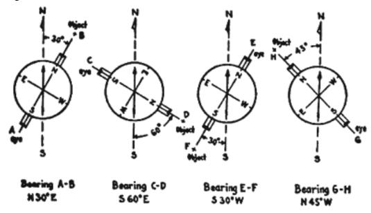
Illustration: Method of Reading Bearings
