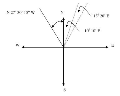
Current magnetic bearing =  $N 27^0 30' 15'' W + (13^0 20' E - 10^0 10' E)$ Current magnetic bearing =  $N 27^0 30' 15'' W + 3^0 10' E$ Current magnetic bearing =  $N 30^0 40' 15'' W$
