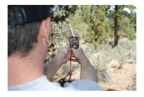
By holding the compass this way, you can use your fingers to easily turn the calibrated dial and line up the arrows to read direction/bearing.
