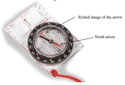
The correct bearing is obtained by turning the calibrated dial until the north arrow (red arrow) is lined up inside the etched image of the arrow.
