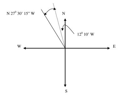
The property line lies N  $27^0$  30' 15" W of the magnetic declination True bearing = N  $27^0$  30' 15" W + N  $12^0$  10' W True bearing = N  $39^0$  40' 15" W
