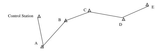
Disadvantage: There are no quick error checks on an open traverse. Best procedures are to measure all lengths multiple times to validate lengths and to read back sights with all foresights to validate direction.
