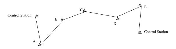
The advantage of the closed polygon is that error checks can be made almost immediately. The expected angle sums are already known and coordinate geometry will give an error check on departures and latitudes (explained later).
