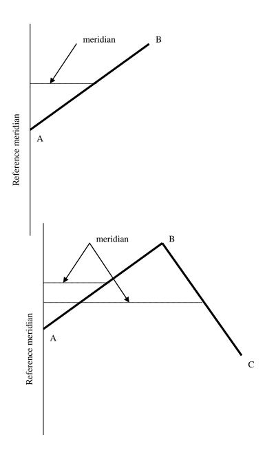
We can calculate the double meridian distance of each traverse line and calculate the traverse area by using the following formulas:
