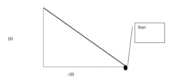
Tan azimuth (or bearing) = departure / latitude Tan azimuth (or bearing) = -10/10
